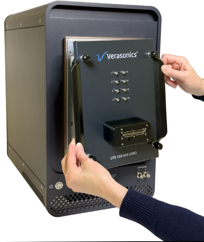
Any UTA can be changed in a few minutes — no tools required
