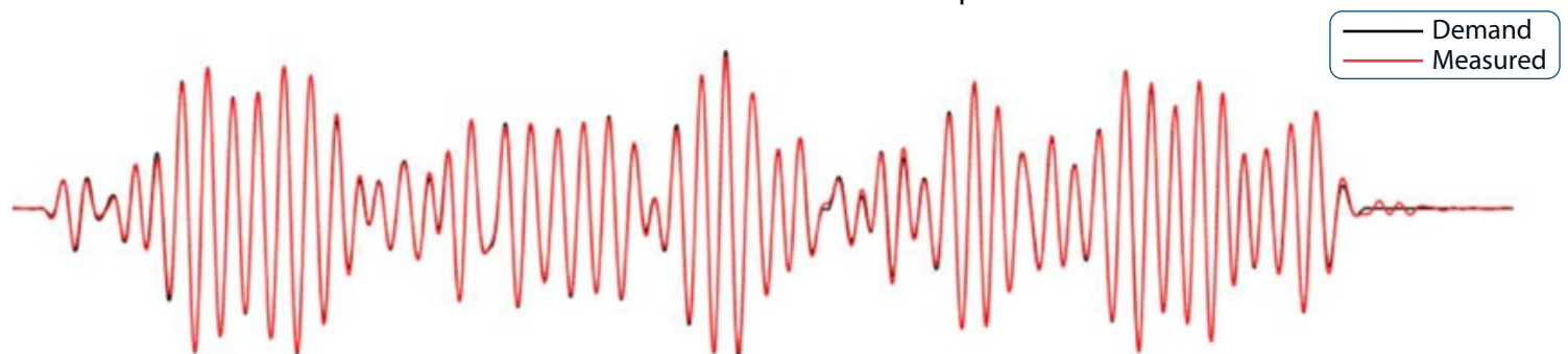
Experimentally measured arbitrary ultrasonic waveform: Pseudo-random 5-11 MHz
