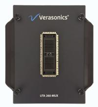
NXT UTA 260-MUX The UTA 260-MUX supports transducers with up to 128 elements on systems with fewer channels.
