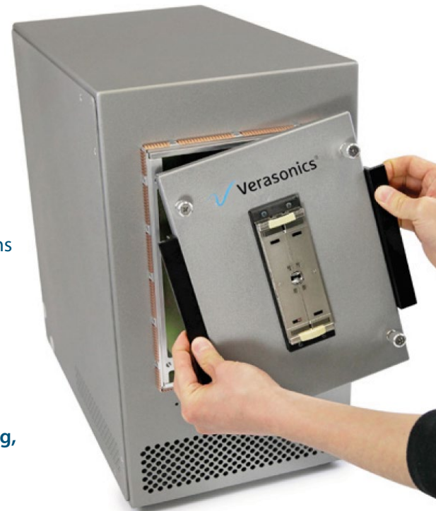
The UTA can be changed in a few minutes — no tools required
