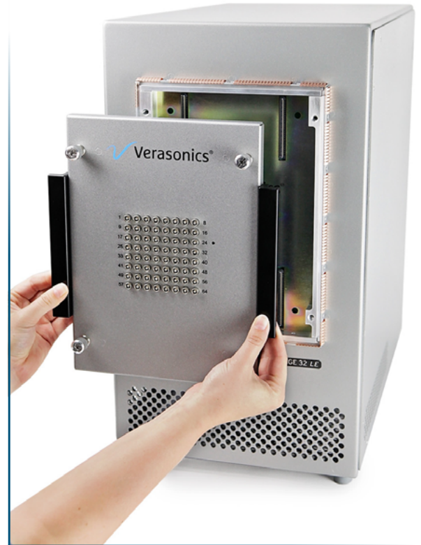
The UTA can be changed in a few minutes — no tools required
