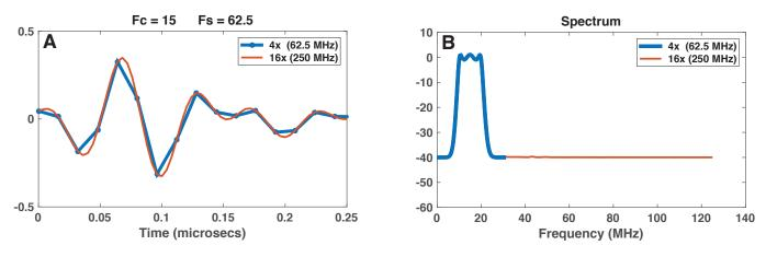
Figure 4. Bandwidth-limited interpolation.
