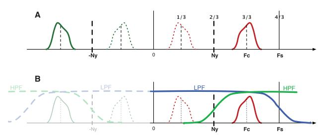
Figure 2. Bandwidth sampling a high frequency signal using a Nyquist limit set below the signal's passband.
