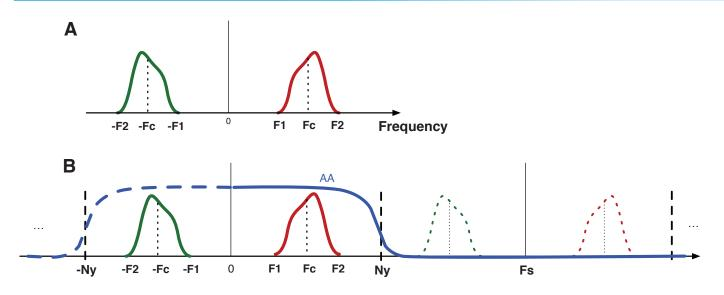
Figure 1. Representation of a signal spectrum, 4x sampling, and the Anti-Alias filter.
