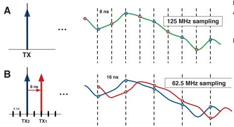
Figure 3. Interleaved sampling using two acquisitions.
