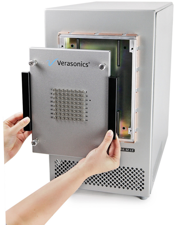
The UTA can be changed in about one minute – no tools required
